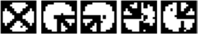
**Fig. 4.** Remaining slopes after removing the subapertures with r.m.s. values outside the valid range.
