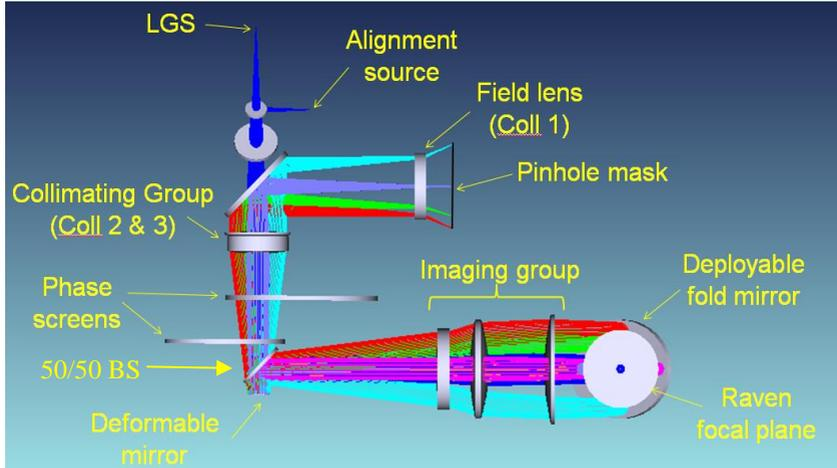
Fig. 3. LGS source, alignment source and optical relay optical systems
