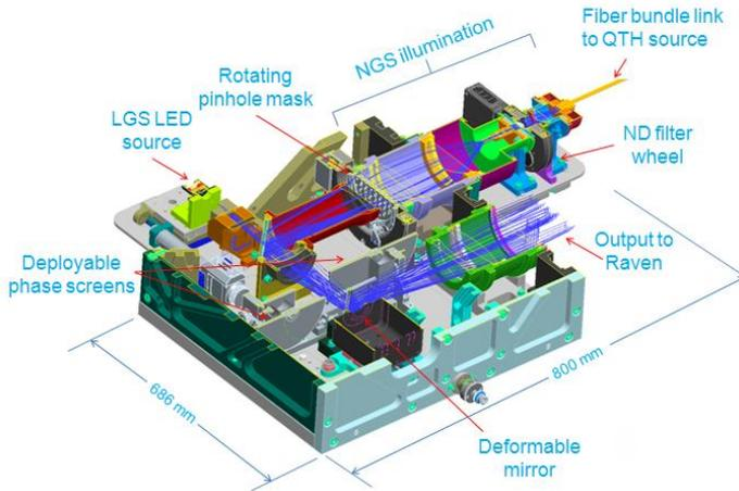
**Fig. 1.** Raven calibration unit opto-mechanical assembly main components
