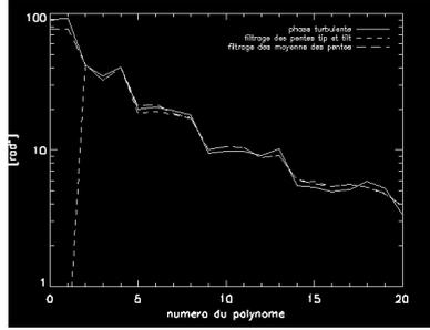
**Fig. 1.** Projection of the turbulent phase onto the Zernike basis(solid line), the filtered phase (long dashed line) and a phase without TTF(dashed line)
