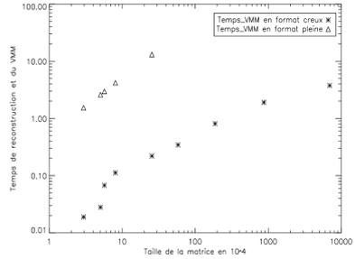
**Fig. 7.** Gain in memory storage and so the calculus time while using sparse matrices.
