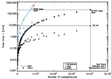
**Fig. 6.** Efficiency of E2E-s comparing to CAOS, where we show the calibration time in terms of sub-apertures.
