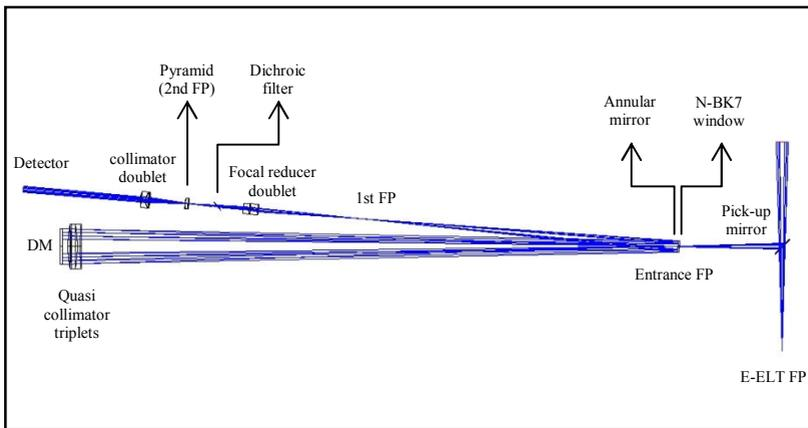
Fig. 1. Optical layout of channel 1.
