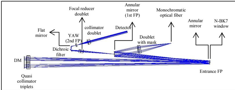
Fig. 4. Optical layout of channel 2.
