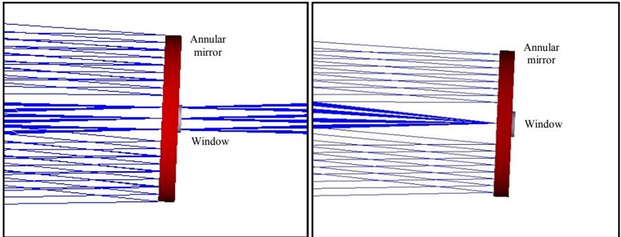
**Fig. 2.** Layout of the N-BK7 window and the annular window. In the channel 1 case (left image), the beam incoming from the telescope (from right to left) pass through the N-BK7 window and has no interference with the beam coming back from the DM (from left to right). In the channel 2 case (right image), the beam incoming from the monochromatic source is reflected by the N-BK7 window towards the DM and has no interference with the beam coming back.
