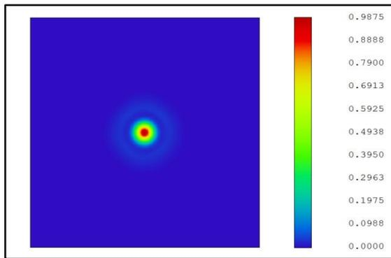
**Fig. 3.** Polychromatic PSF at the pyramid vertex. The theoretical Strehl Ratio is 98.75.
