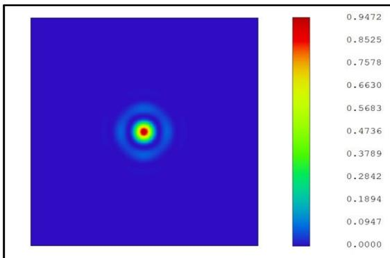
Fig. 5. Monochromatic PSF at the YAW entrance FP. The expected Strehl Ratio is 94.72.
