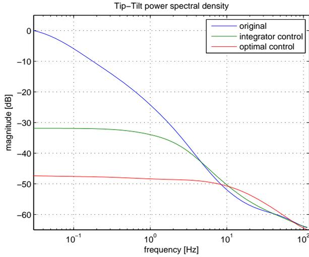
**Fig. 6.** Comparison of simulated control performances in terms of total tip and tilt PSD.
