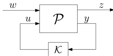
Fig. 1. General system set-up of an  $\mathcal{H}_2$ -optimal control problem.
