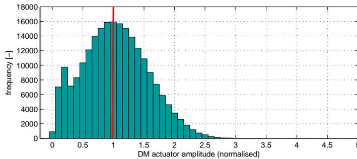
**Fig. 3.** Histogram of required DM actuator amplitudes for optimal control; the red line represents the maximum allowed amplitude.
