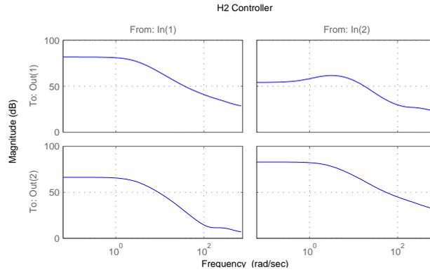
**Fig. 7.** Magnitude of the 2x2 controller frequency response.
