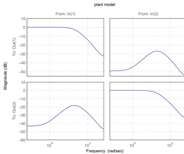
**Fig. 5.** Magnitude of the frequency response of the closed-loop 2x2 tip-tilt system.
