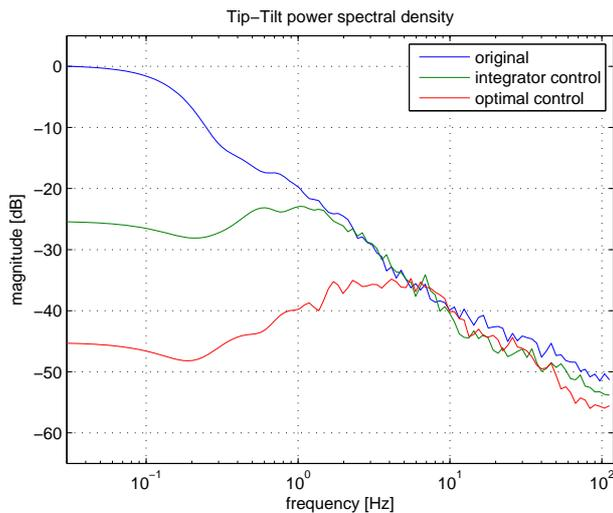
**Fig. 8.** Comparison of on-sky control performances (averaged over several tests) in terms of total tip and tilt PSD.
