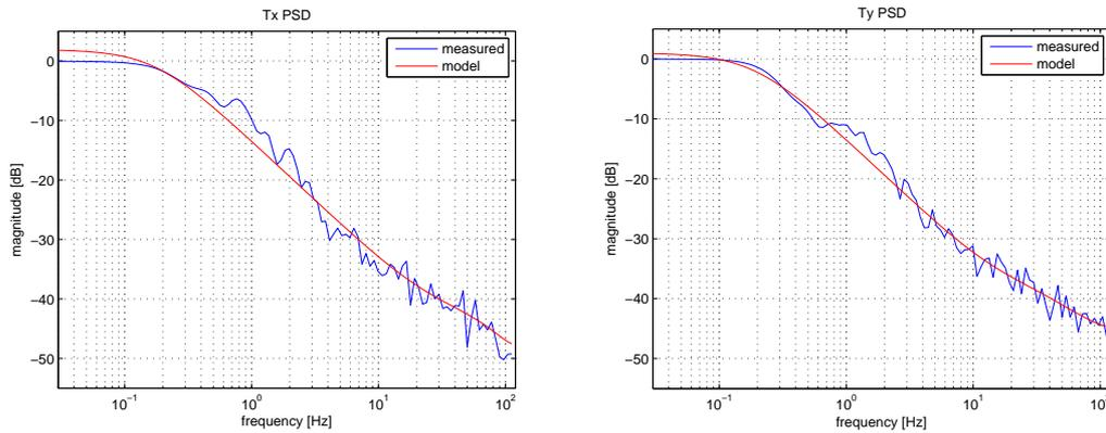
**Fig. 4.** Power spectral density of tip and tilt modes.
