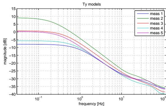
**Fig. 9.** Frequency responses of disturbance models for  $T_y$ .
