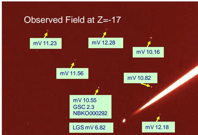
**Figure 9:** typical 5sec exposure CCD image of the LGS, the uplink beam and the magnitude calibration stars, obtained during the commissioning runs at AVSO. The colour table is saturated to show the stars of faintest magnitude detected. The LGS V-magnitude in this frame was  $m_V=6.82$ , with the laser emitting circularly polarized light and the  $D_{20}$  line. The field of view is  $10.56' \times 7.11'$
