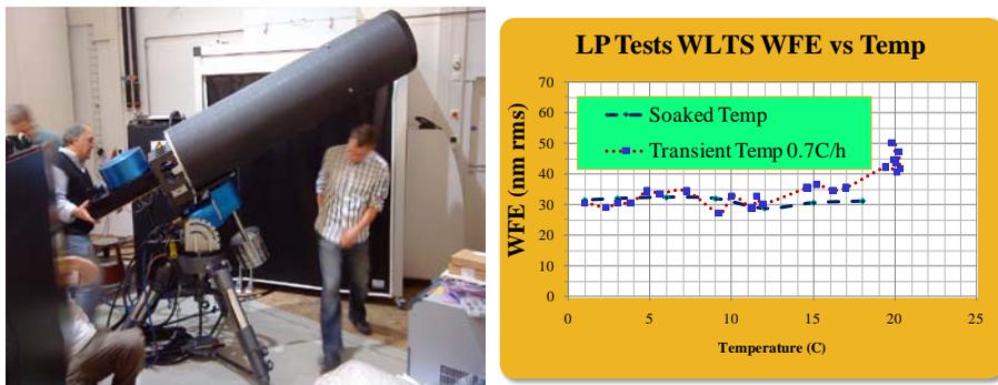
**Figure 6** left: the transportable WLGSU installed on a tripod. The Launch Telescope System has been tested in the climatic chamber for soaked air temperatures and transients. Right: the rms wavefront error of the launch telescope has been tested at different temperatures, showing a good athermalized system and the fulfilment of the specifications (70nm rms)
