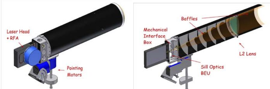
**Figure 4:** Layout of the Wendelstein Laser Guide Star Unit, hosting the 20W laser head and the launch telescope. The telescope tube and interface is in carbon fiber, with a coefficient of thermal expansion chosen to athermalize the lens system focus. The overall weight of the launch telescope + laser head is <85kg. The launch telescope and the pointing motors NTM-500 are from Astelco GmbH.
