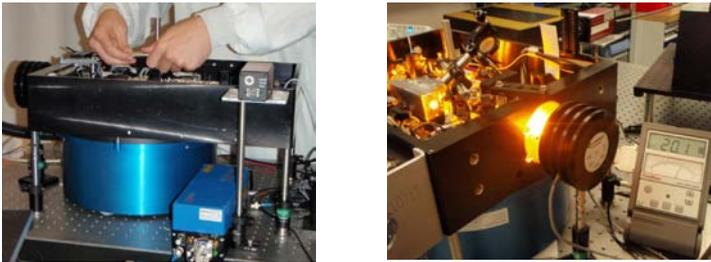
**Figure 5:** the laser head (left) has been integrated and tested together with the company Topica Photonics. The Raman Fiber Amplifier is the blue cylinder attached below the laser head. The 20W power emission is shown in the right picture, taken after the exit window, with the laser head open.
