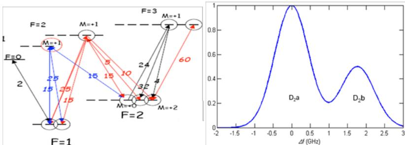
**Figure 3:**  $D_{2b}$  repumping is used to re-inject electrons which have landed in the sodium orbital energy hyperfine ground state  $F=1$  (corresponding to the  $D_{2b}$  line) into the  $F=2$  level, corresponding to the more effective transitions of the  $D_{2a}$  line
