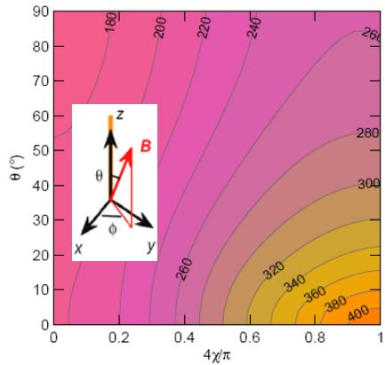
**Figure 1:** contour plot of  $\psi$ , the sodium atom return flux per solid angle, with units  $\text{ph/s/sr}/(\text{W/m}^2)$  vs the Poincaré Sphere angle  $\chi$  in abscissa ( $0 =$  linearly polarized,  $\pi/4 =$  circularly polarized) and the field vector angle  $\theta(\mathbf{B}, \mathbf{S})$  in ordinate, for the case of magnetic azimuth  $\Phi = 90^\circ$  and  $I = 46 \text{ W/m}^2$  (see [1] for details)
