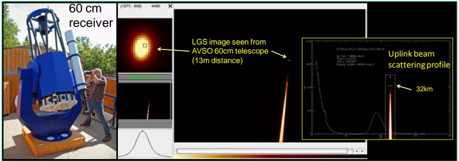
**Figure 8:** Using the SBIG camera on the AVSO 60cm receiver telescope (left) we acquired sky images containing the LGS, the uplink beam and calibrator stars for the photometry.
