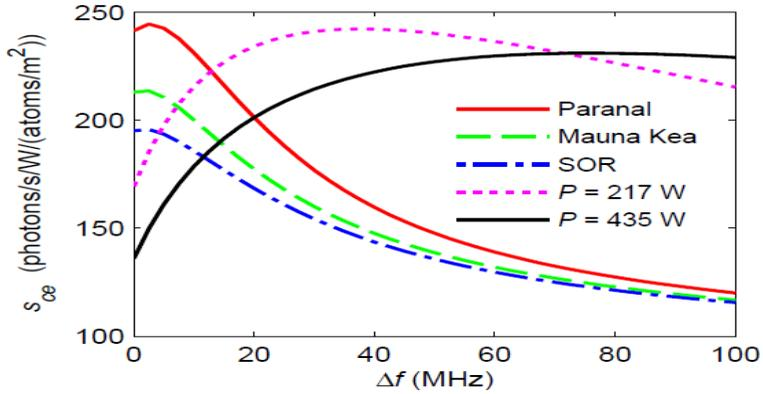
**Figure 2:** Beam efficiency  $s_{ce}$  as a function of laser line FWHM (abscissa) for  $P=20W$  laser at Paranal (solid red curve, standard conditions), Mauna Kea (dashed green), and SOR (dash-dotted blue), depending on the local geomagnetic-field strengths ( $P=20W$ ,  $\theta = \pi/2$ ). Dotted magenta (solid black): CW laser at Paranal with powers of  $P = 217 W$  ( $P = 435 W$ ), possibly representative of microseconds long pulses peak powers. (see [1] for more details)
