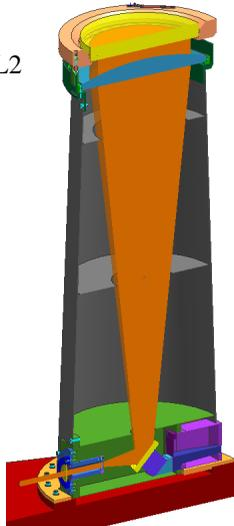
Fig. 4. Concept 1 – CFRP tube
