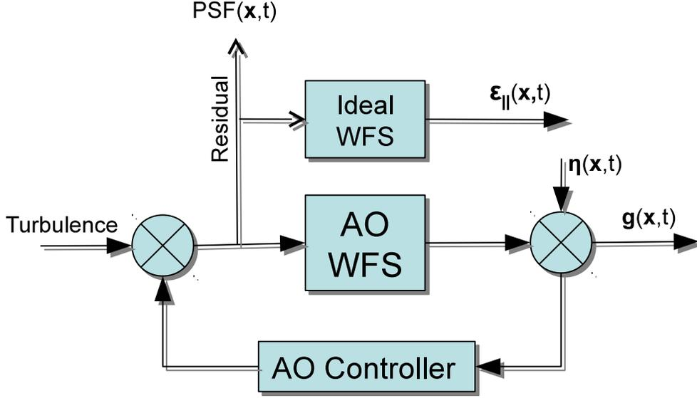
**Fig. 1.** Simplified scheme of PSF reconstruction with the AO WFS affected by measurement noise and aliasing and an ideal WFS that would give direct access to the residual phase after AO correction, here  $\epsilon_{||}(\mathbf{x}, t)$ . For the other variables, see text below.
