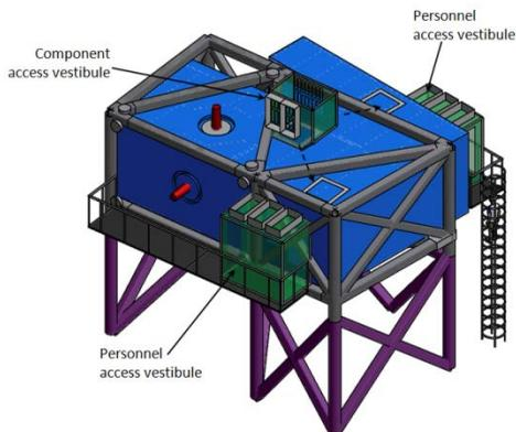
**Fig. 6.** Access to optics enclosure
