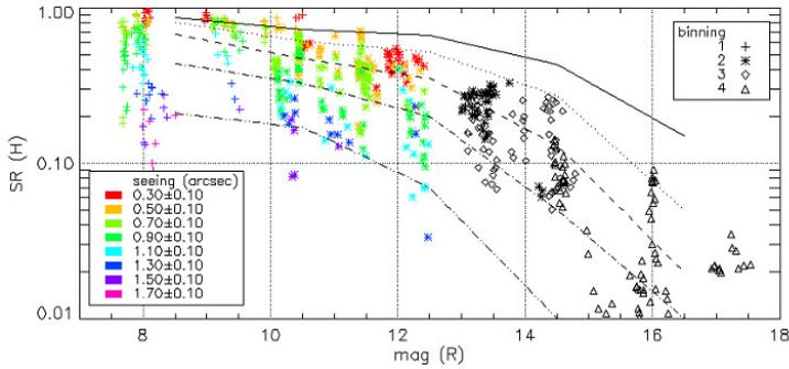
**Figure 2.** The plot reports the achieved SRs in H band as a function of the reference star magnitude. The color of the different points gives an estimate of the seeing values. Note that some of values are underestimated. The different lines refer to simulated performance for seeing values of 0.6, 0.8, 1.0, 1.2, 1.5 arcsec respectively.
