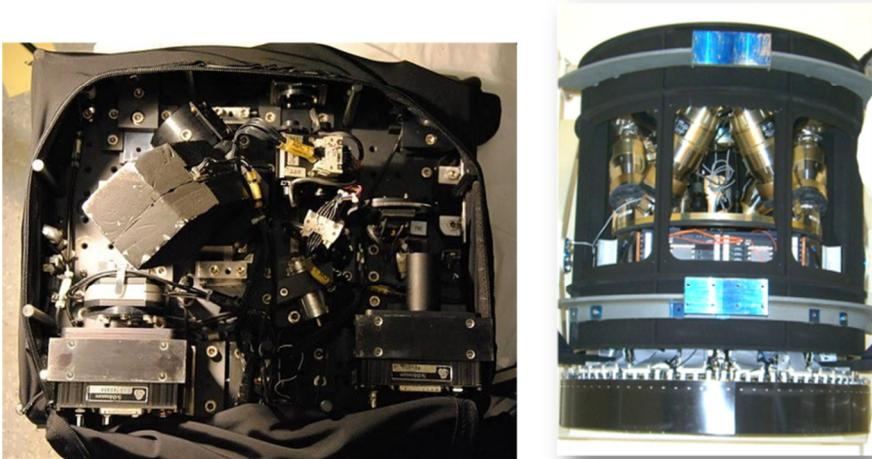
**Figure 1.** A picture of the FLAO system WFS board (left) and of the ASM unit (right).
