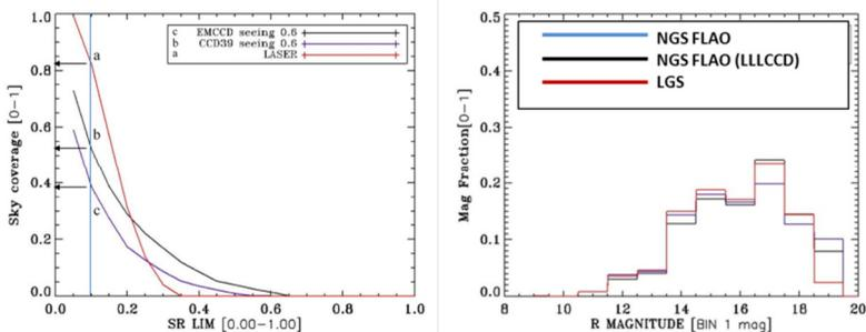
**Figure 5** (left) the sky coverage achieved as a function of the required SR values. A, b and c lines refer to the FLBT AO, the LBT AO upgraded with an EMCCD and a laser system. The laser data are in agreement with results achieved at Keck telescope. (right) Magnitude of the reference star used in the computations for the three systems.
