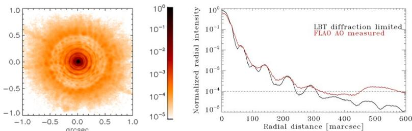
**Figure 4 (Left) The high order corrected LBT PSF in H band. Several diffraction rings are seen plus the external AO control radius. (Right) The radial profile of the image showing a contrast better than  $10^{-4}$ . Such a contrast is achieved without any coronagraph.**
