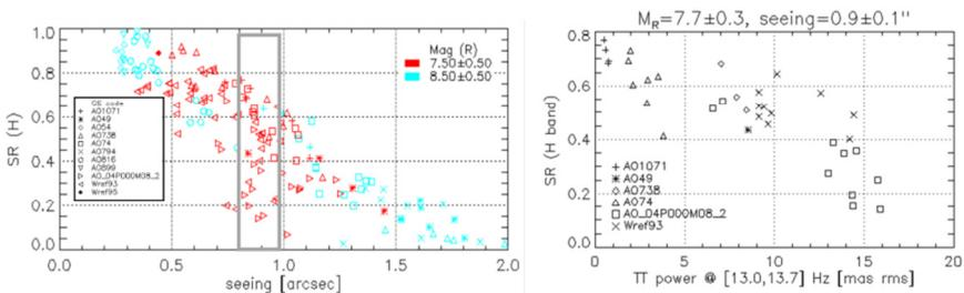
**Figure 3.** (Left) SR versus seeing for star magnitudes between 7.0 and 9.0. (Right) Effect of telescope vibrations on the measured SRs.
