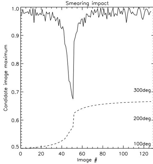
**Fig. 3.** Maximum of an off-axis source during the sequence. Values are normalized to the unsaturated on-axis PSF. The dashed line gives the angle to north of each image in degrees (scale on the right).
