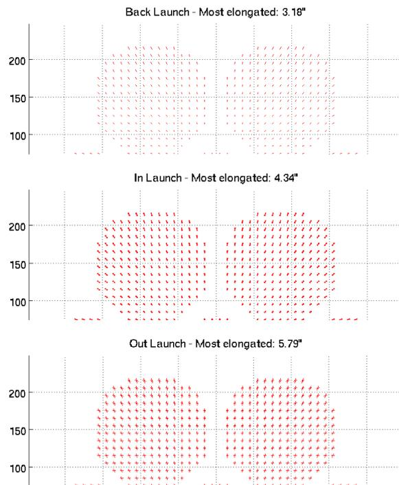
**Fig. 4.** LGS WFS spot elongation for one launch telescope on the back of the ASM, LGS WFS spot elongation for six launch telescopes within the segment primaries and LGS WFS spot elongation for three launch telescopes on the primary segment edges
