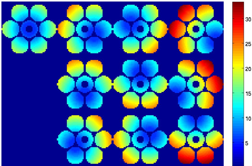
**Fig. 5.** LGS WFS noise maps for the 3 launch telescope configuration.
