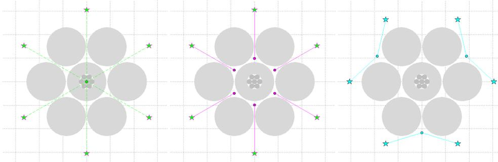
Fig. 3. 6 lasers launched from the back of the ASM, 6 launch telescopes within the primary segments and 3 launch telescopes on the primary mirror edges.
