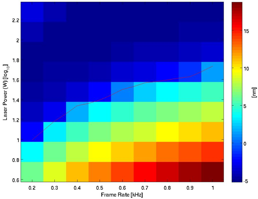
**Fig. 7.** Difference between the central and edge Laser launch WFS measurement error versus the Laser power and the frame rate.
