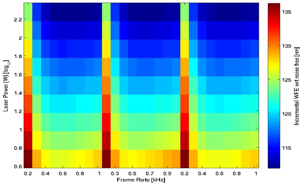
**Fig. 6.** LGS WFS measurement error for the 3 configurations versus the Laser power and the frame rate.
