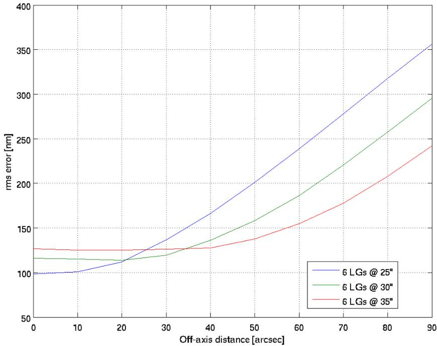
Fig. 2. Tomographic error as a function of the off-axis distance for 6 LGS at different radii.
