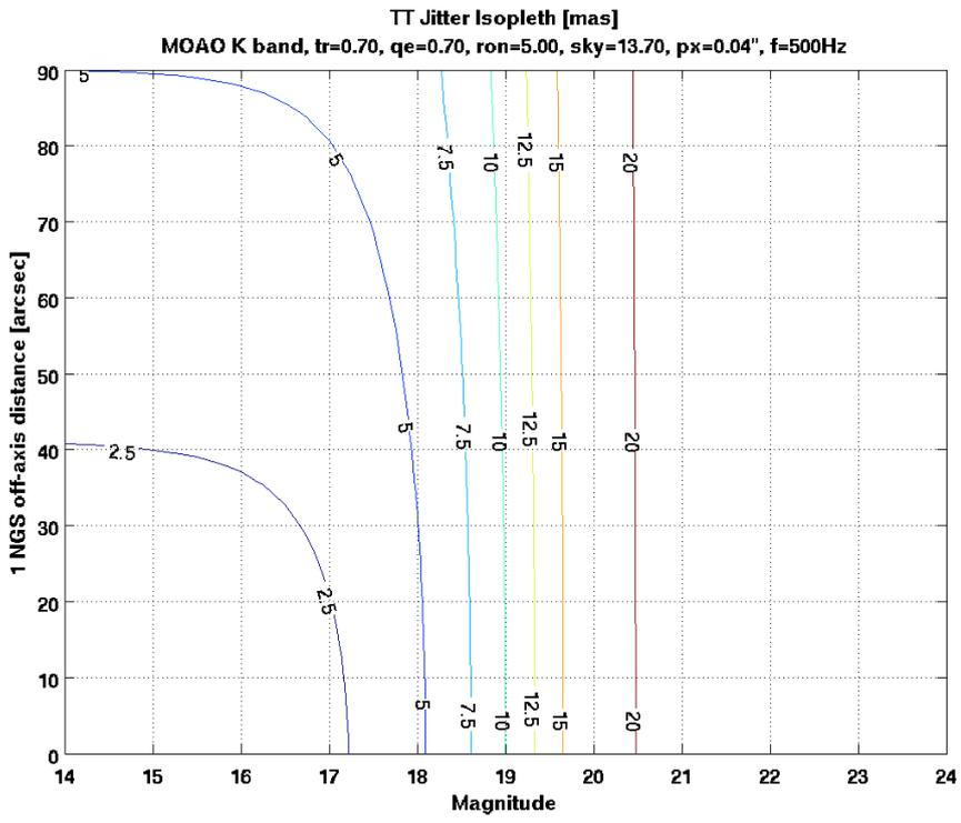
Fig. 11. Tip-Tilt Tomography with 1 AO corrected K band TT star.
