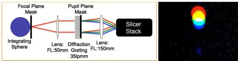
**Fig. 2.** Right: Cartoon depicting our pre-optics setup that creates our single ‘simulated’ speckle. Left: RGB image taken at the location of the slicer stack, after the pre-optics, showing our speckle as the diffraction limited point source that is moving with wavelength.
