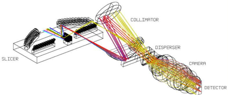
**Fig. 1.** Schematic view of the SWIFT slicer spectrograph that was used for this experiment.
