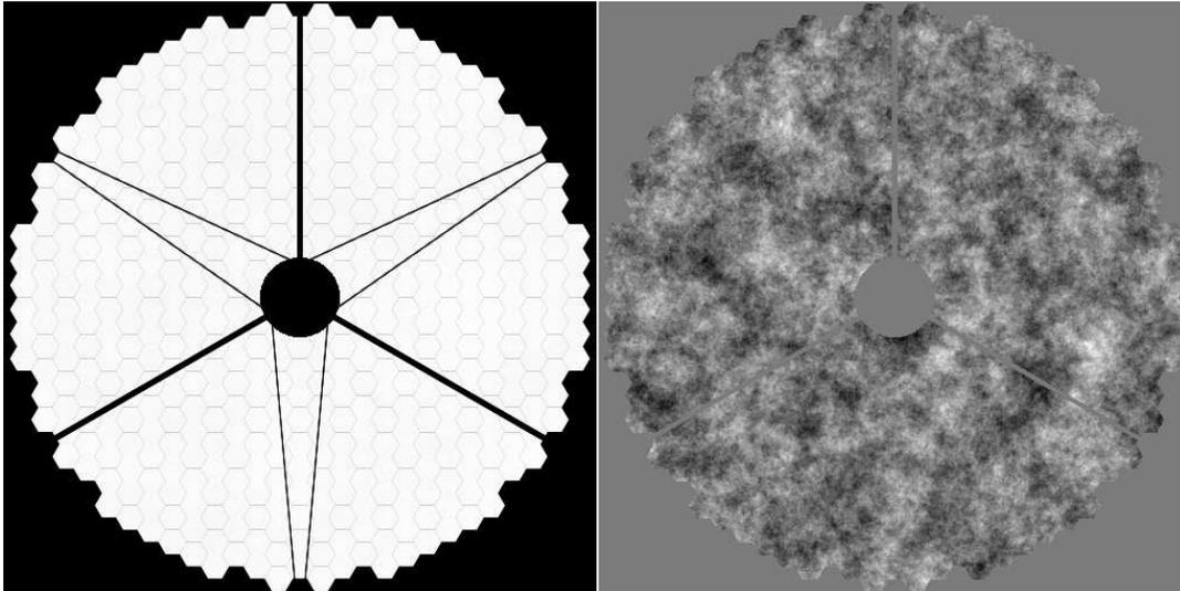
**Fig. 1.** The simulated TMT M1 mirror (left) and its static phase aberration (right). Independent segment aberrations were not simulated since they were generating issues with the basic wavefront sensing algorithm used for the simulation presented in this paper (see below).
