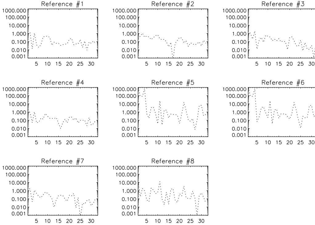
**Fig. 6.** Wavefront error as a function of Zernike coefficients for different reference. The number corresponds to the reference listed in 3. The graph shows results with the TMT configuration, 500 photons and a readout noise of 3 electrons.
