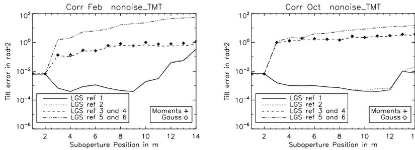
**Fig. 3.** Total tilt error in  $\text{rad}^2$  (i.e. considering both axis) as a function of the subaperture position, for different references. The centroid method is the correlation and there is no noise. The left graph corresponds to a profile in February and the right graph from October.
