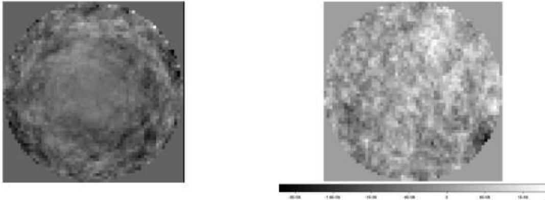
**Fig. 5.** Reconstructed wavefront without noise (left) and with noise (right). The graphs show results for the TMT configuration and with noise (we used 500 photons and a readout noise of 3 electrons).
