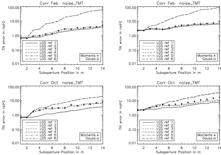
**Fig. 4.** Total tilt error in  $\text{rad}^2$  as a function of the subaperture position, for different references. The centroid method is the correlation and we considered two levels of noise. The graph on the left corresponds a noise level of 500 photons and no readout noise and the graph on the right corresponds a noise level of 500 photons and a readout noise of 3 electrons. The top row shows results from February and the bottom row shows results from October.
