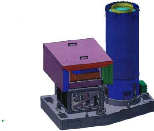
**Fig. 4.** LTS without Cover and Baffle. The OTA is to the right. On top of the BCDS (to the left) the Laser Head is installed. The Laser Head output beam is entering the BCDS vertically from the top. The LTS Baseplate hosting the Laser Head, BCDS and OTA is installed on the UT4 Centrepiece using three tilt adjusters and can be removed and re-installed without re-alignment.
