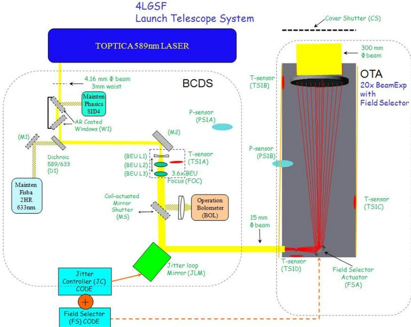
**Fig. 3.** Schematic layout of the LTS with BCDS (left) and OTA (right). Note also in parenthesis the acronyms assigned to the different LTS components. Note that in this layout the quarter-wave plate element at the OTA entrance to produce the output circular polarization is not shown.
