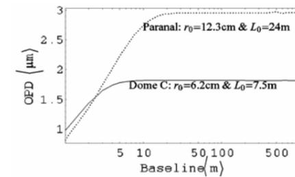
OPD versus baseline for an interferometer of 1m telescope diameter in the case of typical conditions of Dome C and Paranal.
