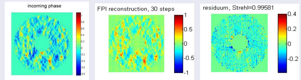
Reconstruction from the full nonlinear model [2] via FPI with 30 steps, the mean restoration is done over the square. From left to right: the incoming phase, the reconstructed phase, the residual. Sampling over the subapertures is not considered.
