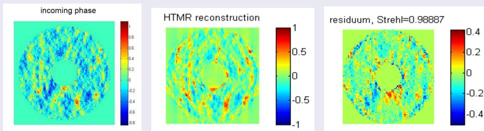
MATLAB based HTMR reconstruction of the masked phase from the full nonlinear model [2]. From left to right: the incoming phase, the reconstructed phase, residuum and Strehl ratio. Mean restoration is done over the square. Sampling over the subapertures is not considered.
