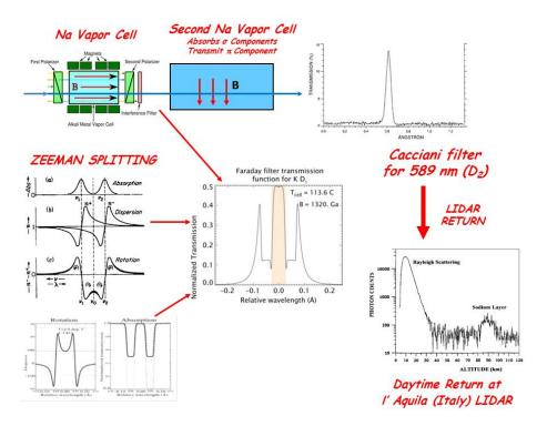
**Fig.** 1. Diagram explaining the working of the Magneto-Optical Filter for Na-lasers. Note that the second Na vapor cell may be omitted for the present application
