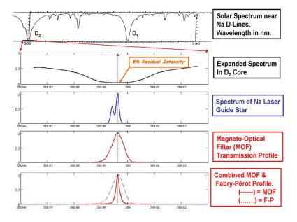
Fig. 2. Spectrum distribution of day sky, Na D2-LGS and filter transmission.
