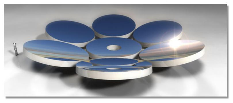
Gregorian optical configuration Seven 8.4 m primary mirror segments (2 optical prescriptions) Seven 1.05 m secondary mirror segments (2 optical prescriptions) 25.4 m edge-to-edge; area equivalent to 21.9 m diameter circular aperture
