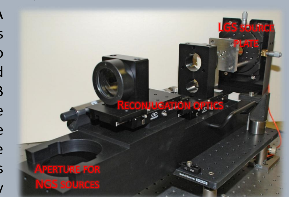
LGS source path during assembly and testing at the UKATC. The system will be ultimately mounted vertically in the Telescope Simulator.
